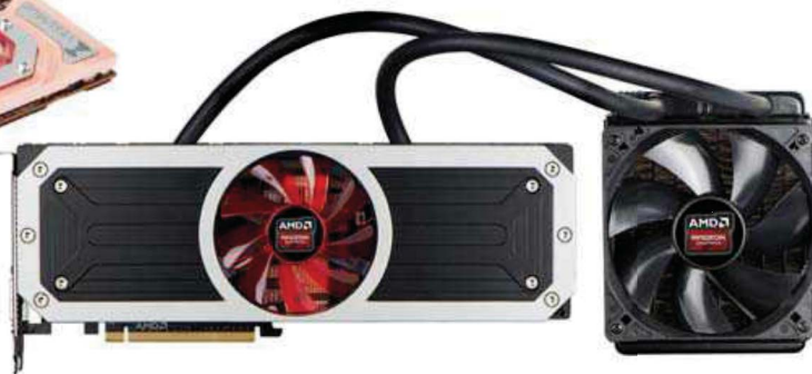
AMD Radeon R9 295X2公版水冷模块
