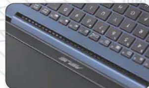
● 散热孔被安置在转轴内侧
