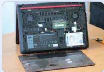
● 拧下一颗螺丝即可拆下底盖
