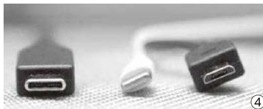
• USB-C、Lightning和MicroUSB接口对比
