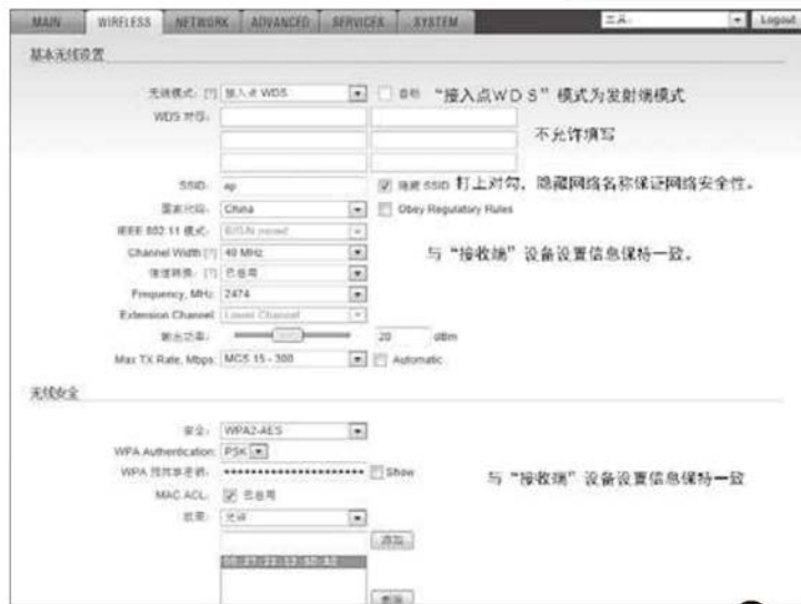
无线网桥发射端“WIRELESS”配置
