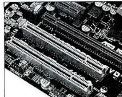
PCI-E×16, PCI-E×1, 2×PCI的设计,扩展性只能说中规中矩
