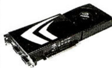
NVIDIA GTX260显卡，正反面各7片显存，共32bit×14 = 448bit
