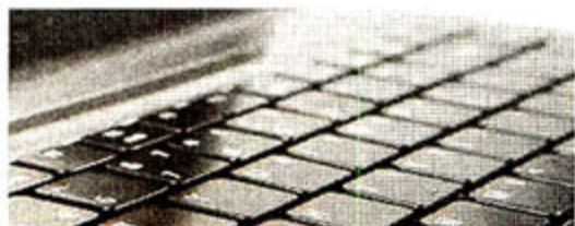
▲同3810T/4810T一样,这款4810TG同样采用悬浮式巧克力键盘,按键偏硬,但键程较长,敲击感上佳
