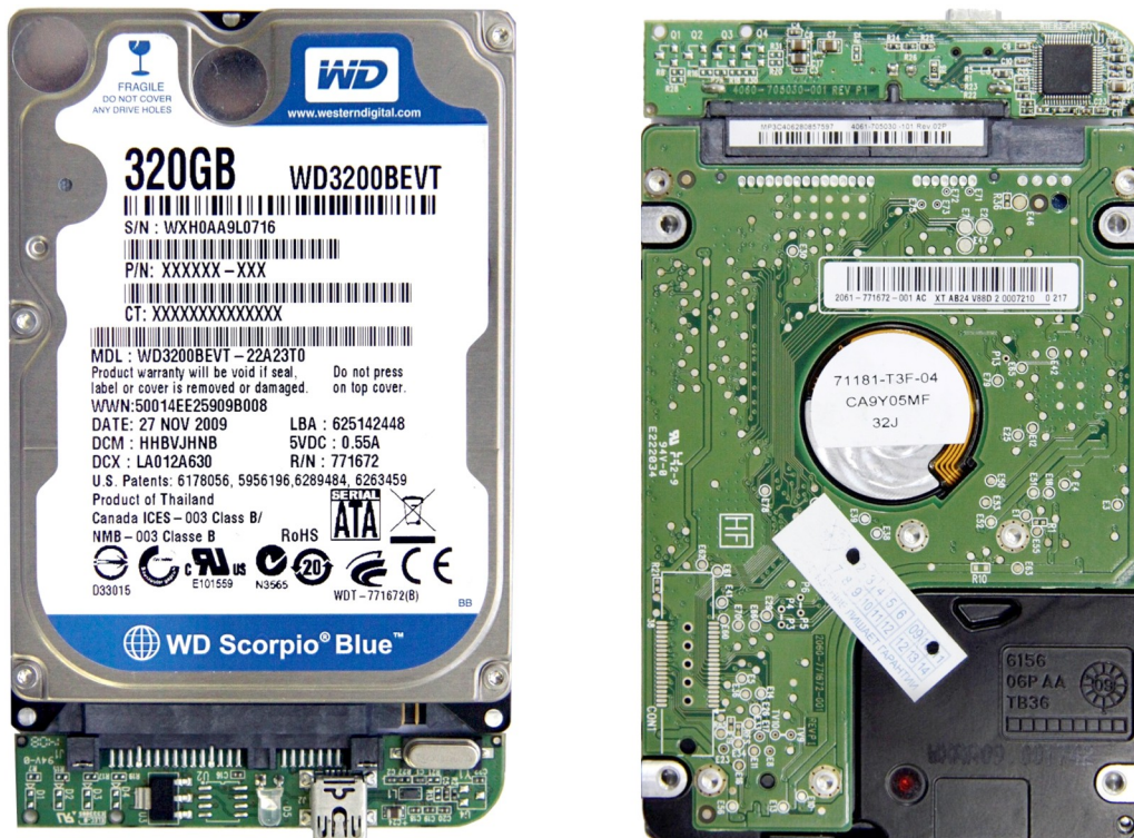
Fig. 2.3. WDC Marvell SATA HDD connected using the SATA - USB adapter.
