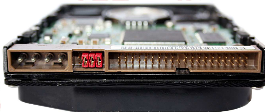
Fig. 8.13. Jumper settings on the drive.
