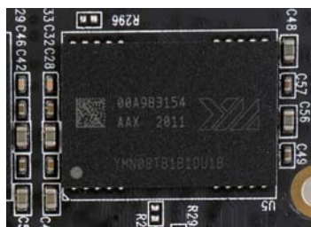
光威弈pro国产固态硬盘采用了Xtacking架构64层TLC 3D NAND闪存
