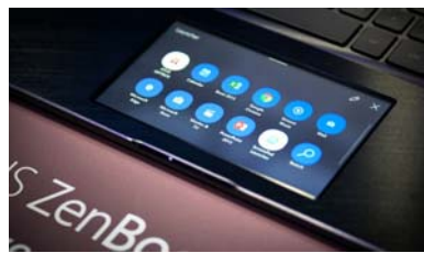
灵耀X Pro的ScreenPad功能,触控板变身屏幕
