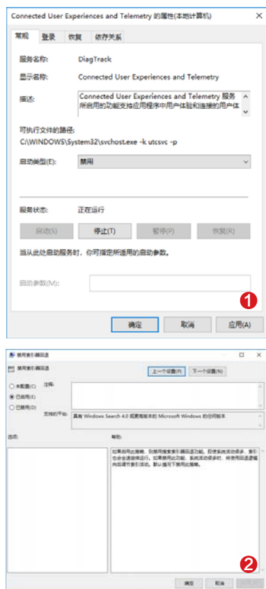
图1: 禁用Connected User Experiences and Telemetry服务。图2: 启用“禁用索引器回退”策略。
