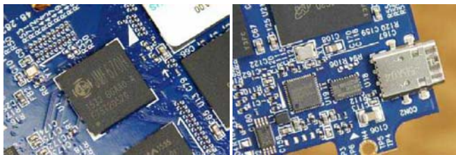
JMicon JMF667H SSD主控与祥硕ASM1351 Type-C主控芯片
