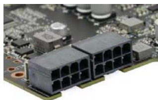
显卡的供电接口变为8pin+8pin
