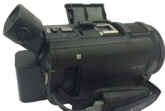
顶部热靴可接拾音器和 AS 200V 摄像机
