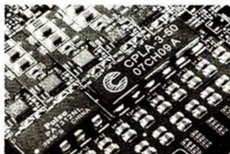
▲ Pulse PA1312NL+CPLA-3-50P耦合电感
