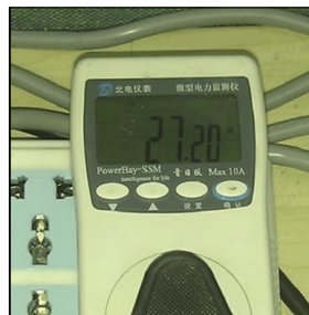
●GPU 满载功耗 27.2W
