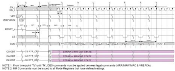
Figure 3 — RESET_n and Initialization Sequence at Power-on Ramping
