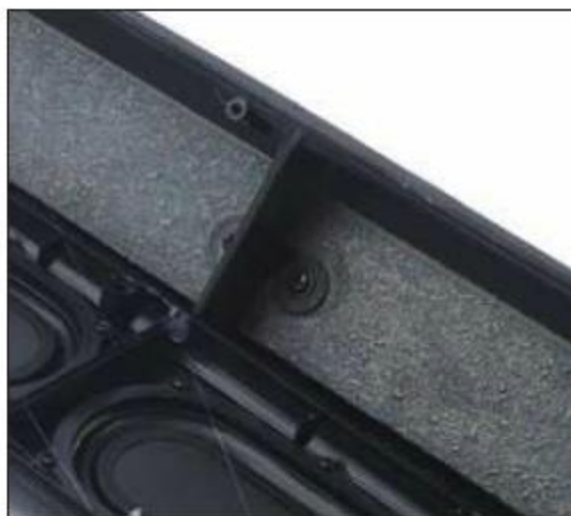
② 箱体内部安置了配重块
