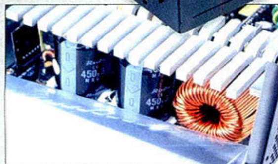
① 两颗主电容采用红宝石MXG 330 \mu F(450V/105 ^{\circ} C)电容
