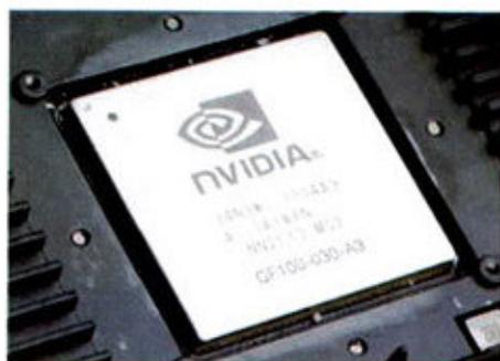
① GeForce GTX 465显卡的核心代号为GF100-030-A3
