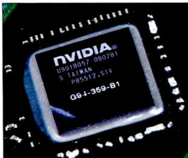
▲ GeForce 9600 GT绿色节能版显卡的核心代号为G94-359-B1
