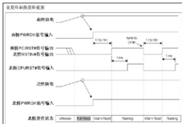
Intel芯片组复位时序和波形(引自Intel I/O Controller Hub 7 (ICH7) Family Datasheet)
