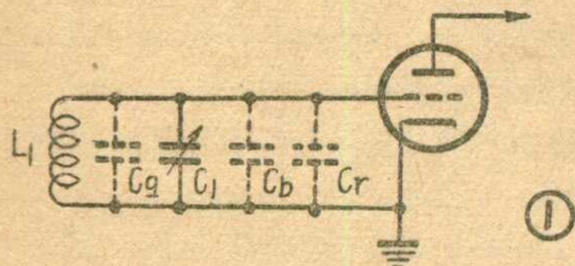
附加电容  $C_0 = C_g + C_b + C_r$
