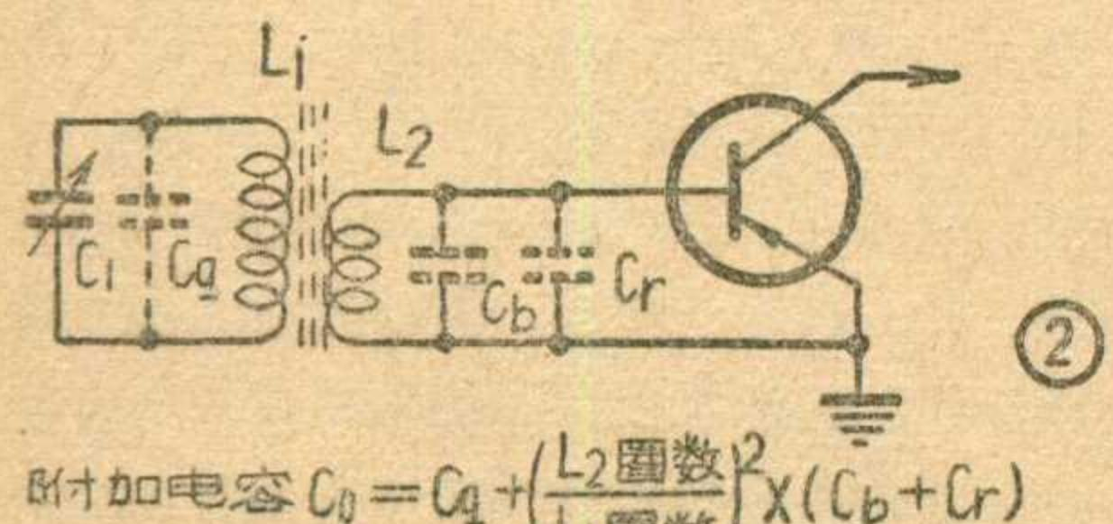
附加电容  $C_0 = C_1 + \left( \frac{L_2 \text{ 圈数}}{L_1 \text{ 圈数}} \right)^2 \times (C_b + C_r)$
